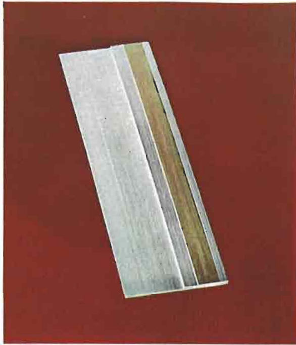
Fig. 5 Many types of connectors incorporate two or more thicknesses of metal in their cross section. The development of profiled bi-metal strip makes it possible to manufacture such parts in a single press operation. This is only one example of a range of profiled strips being produced by Johnson Matthey Metals and comprises an inlay of 10 per cent copper-20 per cent silver-gold in nickel silver
