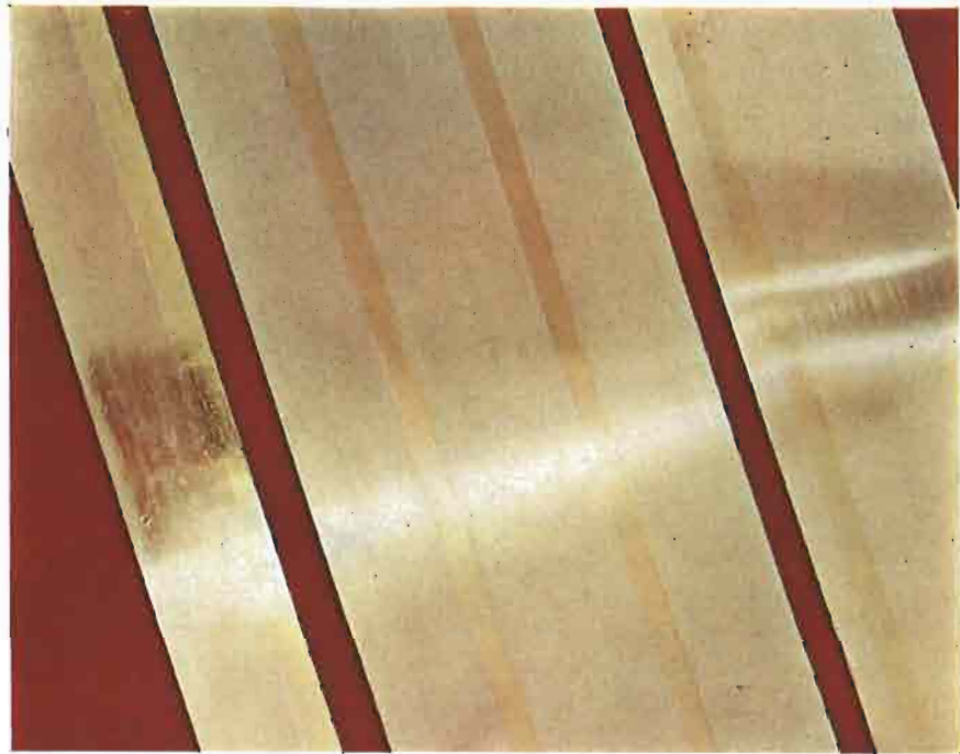
Fig. 2 One means of restricting gold to a required contact area only has been made possible by the production of long coiled strips of phosphor bronze or nickel silver with a stripe of electroplated gold running along its entire length. If necessary, more than one stripe can be produced on one or both faces, as shown in the photograph of strips manufactured by N. T. Frost
