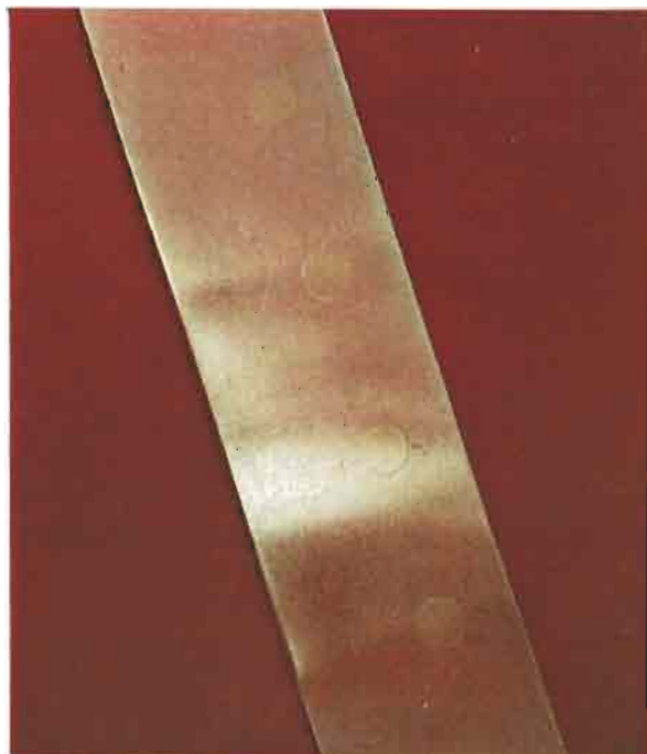
Fig. 3 An alternative method of employing continuously plated strip is achieved by a further development, the production of regularly spaced and accurately located gold plated areas
