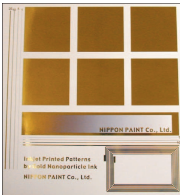
Figure 11 Inkjet Output Pattern using Gold Nanoparticle Ink –High Dot Density–
