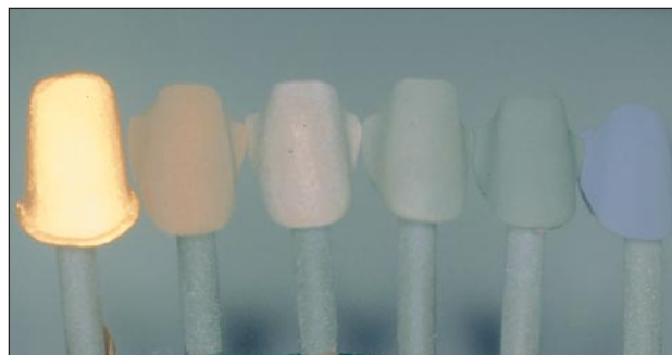
Figure 5 Oxide colours of different dental alloys compared to electroformed pure gold. From the right: titanium, cobalt/chromium; palladium base, two different high gold alloys, electroformed pure gold
